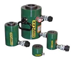
Center hole cylinders are available in both single and double acting styles. These cylinders are primarily used for pushing and pulling applications. Both styles have a center tube that allows a rod or cable to pass through the cylinder and assist in tensioning / pulling applications.
