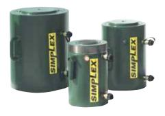
Double acting cylinders are hydraulically driven in both directions. These cylinders are used in many general purpose applications where retraction speed is required or the mechanical forces required for return is not available. This cylinder type requires a pump source with a 4 way valve for proper operation.
