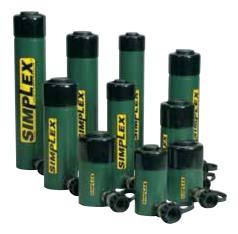
Single acting cylinders are hydraulically driven in one direction. These cylinders are used in many general purpose applications when retract speed is not a requirement. This cylinder type requires a pump source with a single acting valve for proper operation.
